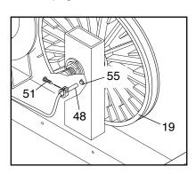
for clarity). Slide the Reed Switch slightly toward or away from the Magnet. Make sure that the Magnet will not hit the Reed Switch. Retighten the Screw. Turn the Pulley (19) for a moment. Repeat until the console displays correct feedback. When the Reed Switch is correctly adjusted, re-attach the left side shield.
